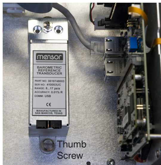
Figure 8.5.3.2 - Internal Barometric Reference
