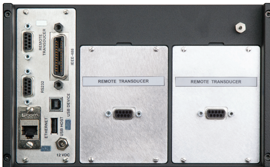
Figure 5.4 B - Two remote transducer interface connections installed
