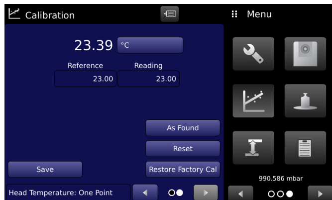
Figure 8.2.6.1-D Saving One Point Calibration
