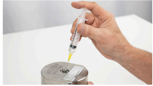
Figure 8.1.2.2.2-D Fill with oil
