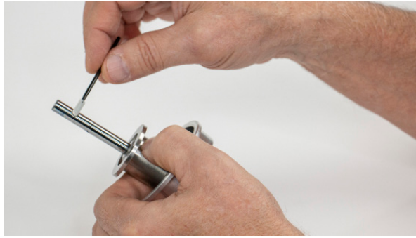
Figure 8.1.2.2.2-C Swab piston with oil
