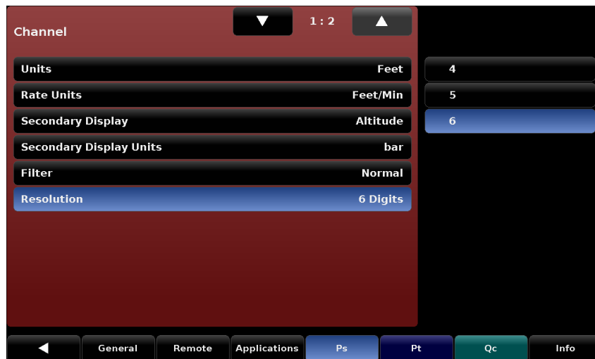
Figure 7.3.6 - Resolution, [Ps] / [Resolution] / [6]
