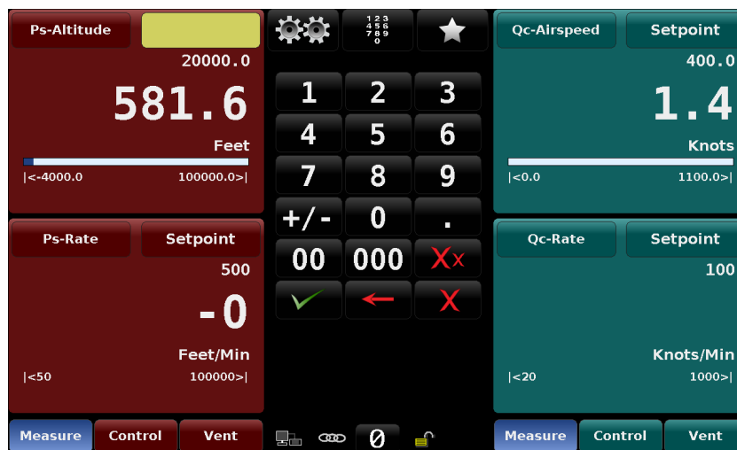
Figure 6.2.4a - Ps Altitude setpoint active (yellow area) - ready for setpoint entry using the number pad.
