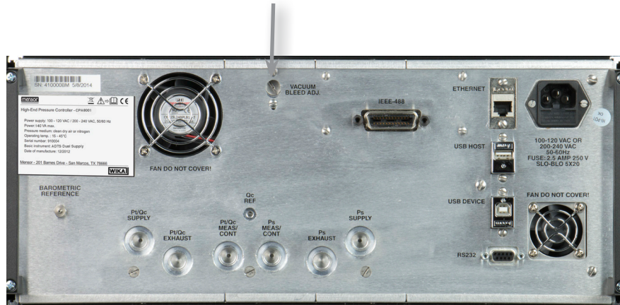
Figure 6.2.14c - Rear Panel with Vacuum Bleed Valve
