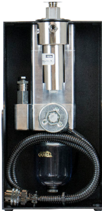
Figure 8.9.2 - Automatic Contamination Prevention System
