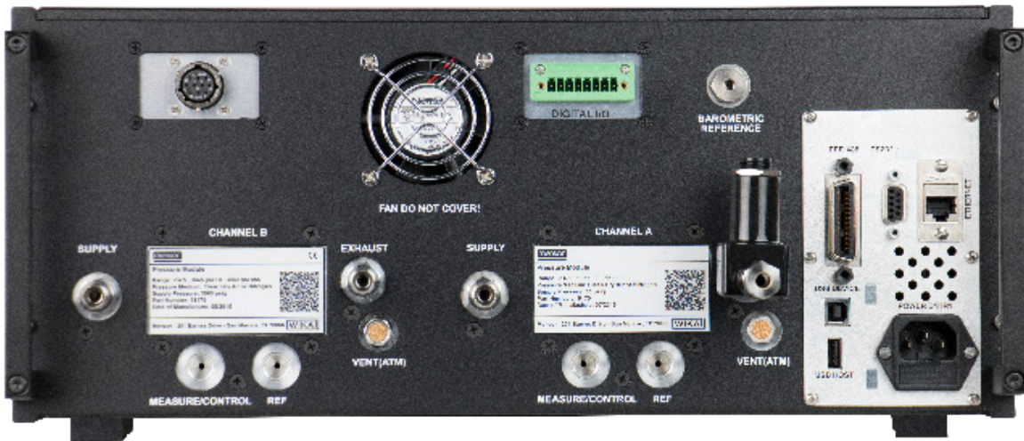
Figure 8.11-A - Vacuum Regulator installed on Exhaust Port
