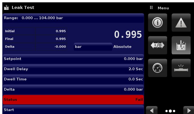
Figure 6.4.12-A Leak Test Fail (left) and Pass (right)
