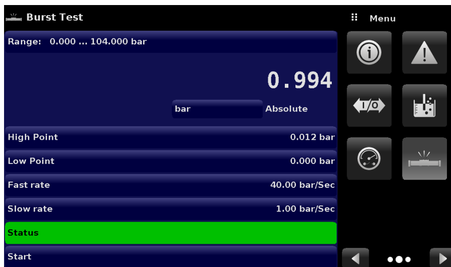
Figure 6.4.14-B Burst Test Complete (No Burst)
