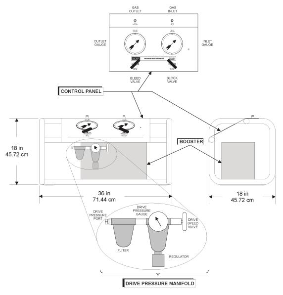
Figure 1 - PBS Mechanical Views (Open Frame)
