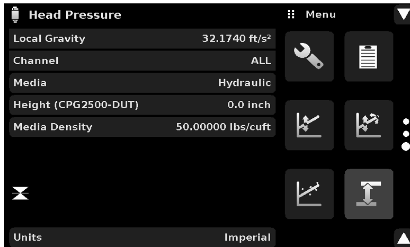
Figure 9.6-D - Head Pressure, Hydraulic
