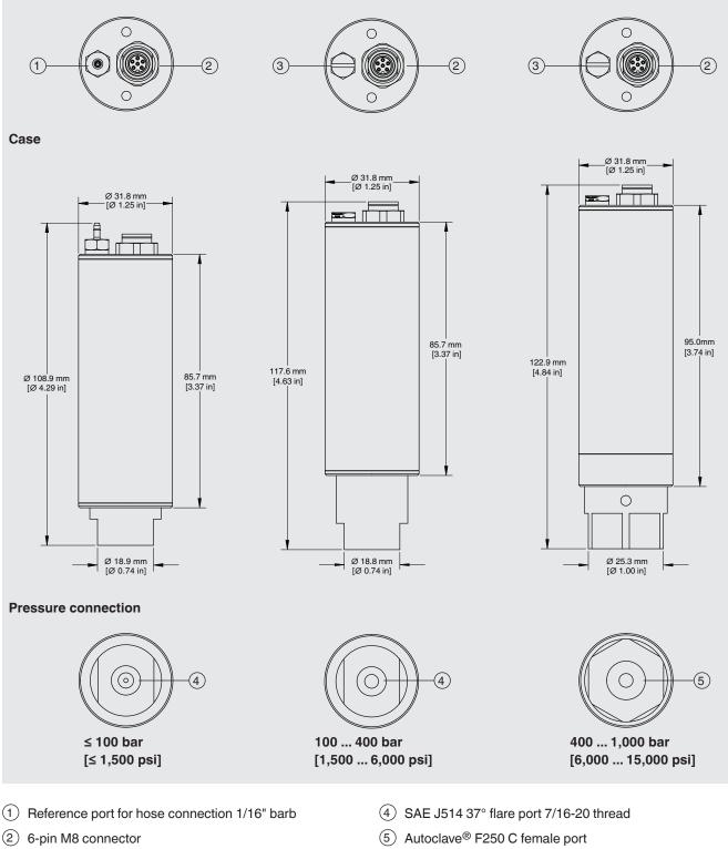
1) Reference port only for gauge pressure range; the port is plugged at absolute pressure range and sealed gauge ranges.
