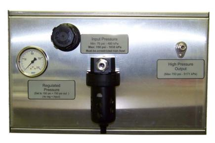
and the regulator knob is not fully counterclockwise. The input regulator filter provides basic filtering of large particles and liquids. It should periodically be checked for excessive contamination and emptied of liquids. **Note: The input pressure supply should have**
