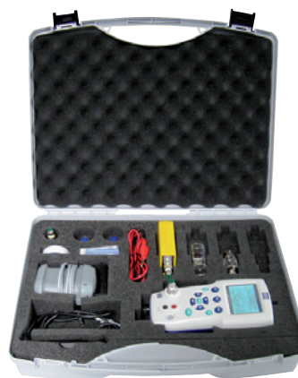
Hand-held pressure calibrator with service case
