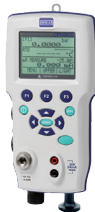
Hand-held pressure calibrator with integrated hand pump
