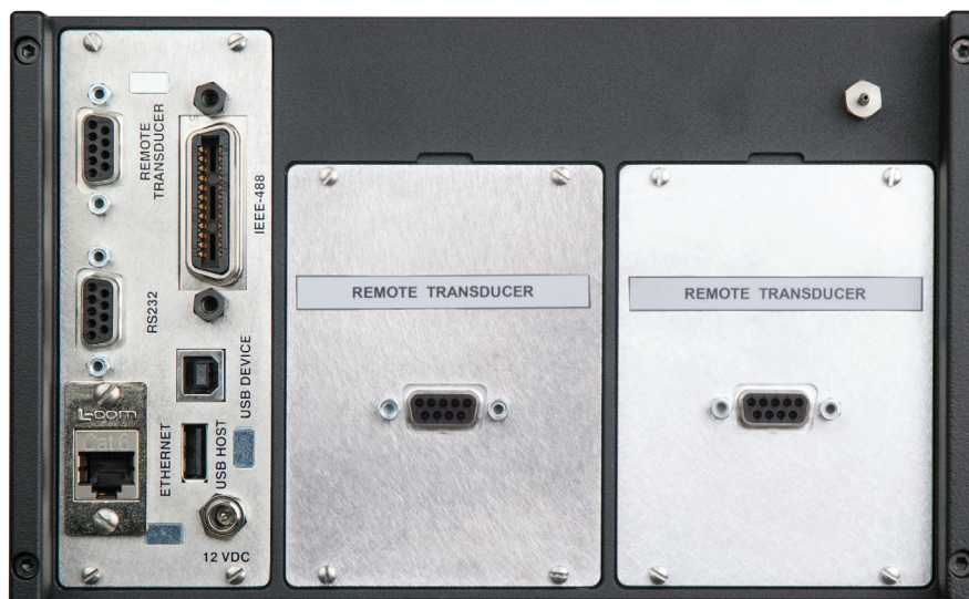
Figure 5.4 B - Two remote transducer interface connections installed
