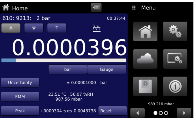
Figure 6.4.1.1-B Unstable Pressure Reading
