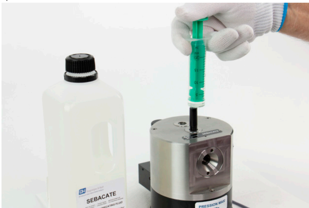
Figure 8.1.2.3.3-A Oil Filling Process
