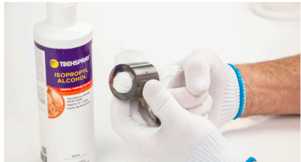
Figure 8.1.2.1.2-A Piston and cylinder cleaning
