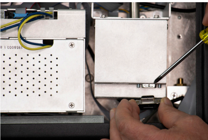
Figure 8.1.4.4-C Unplugging Vacuum Transducer
