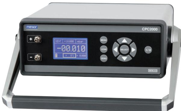
Pressure controller, portable low-pressure version,
