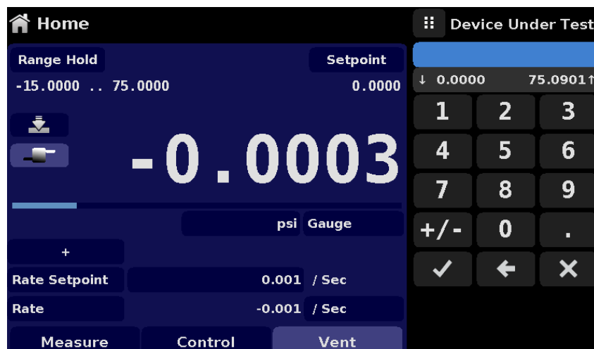
Figure 8.6.3-C - DUT pressure for purge sequence
