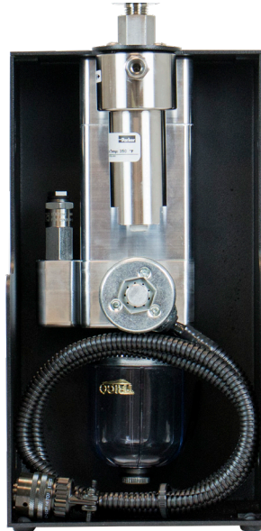
Figure 8.6-A - Automatic Contamination Prevention System
