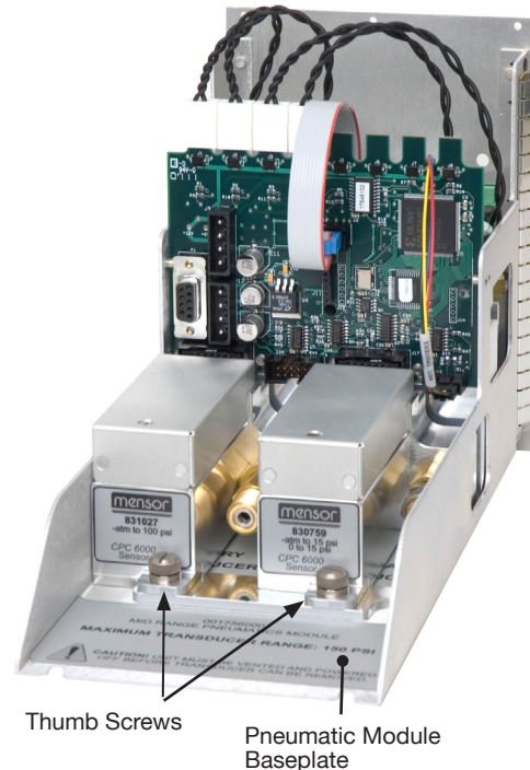
Figure 9.3.1 - Pneumatic Module, Solenoid Valve Regulator
