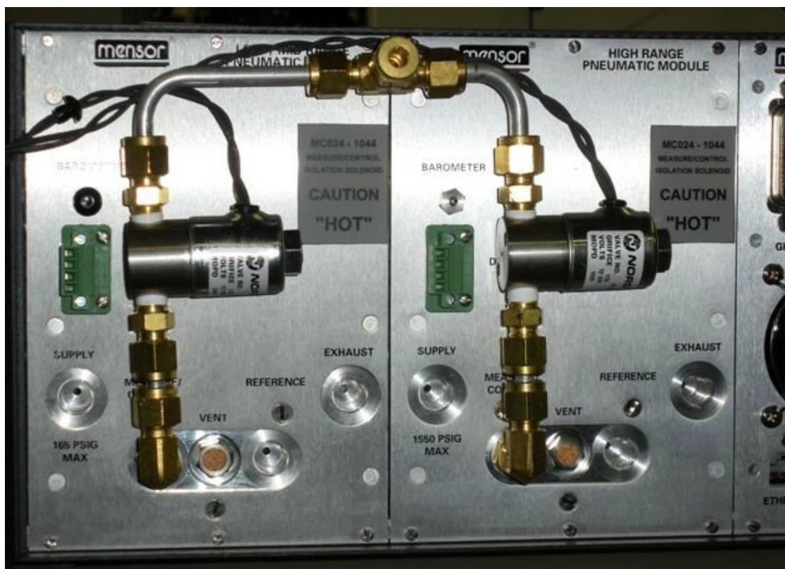
Figure 8.7 - Rear view illustration of plumbing for the Dual Solenoid Single Output Option
