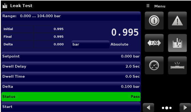
Figure 6.4.12-A Leak Test Fail (left) and Pass (right)
