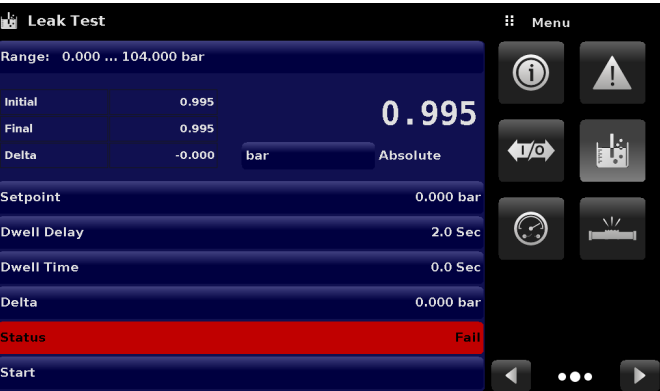
Figure 6.4.12-A Leak Test Fail (left) and Pass (right)
