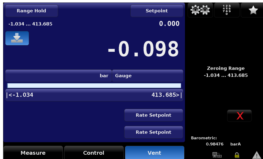
Figure 6.2.14-A Zero Button in Gauge
