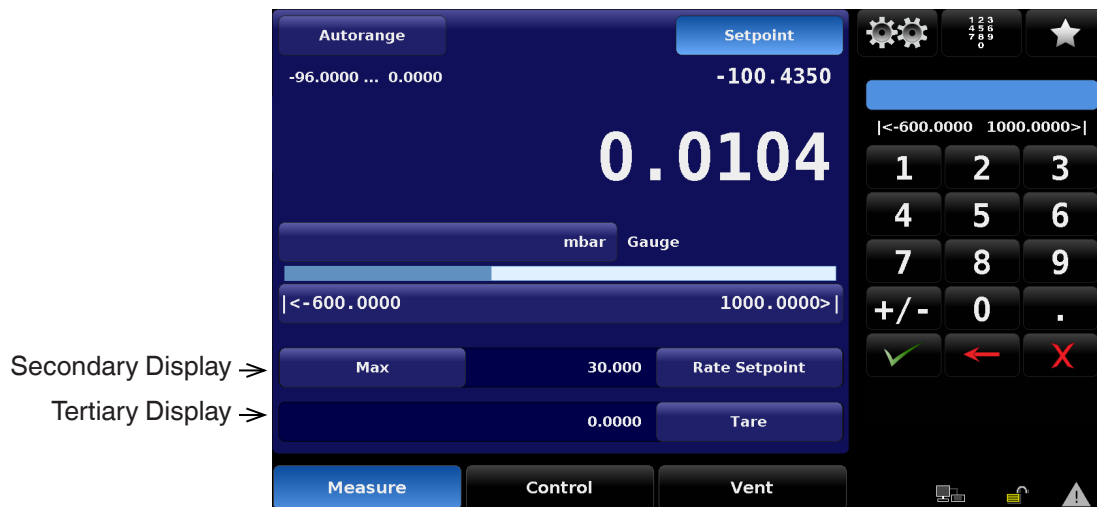
Figure 6.2.9a - Secondary and Tertiary Displays
