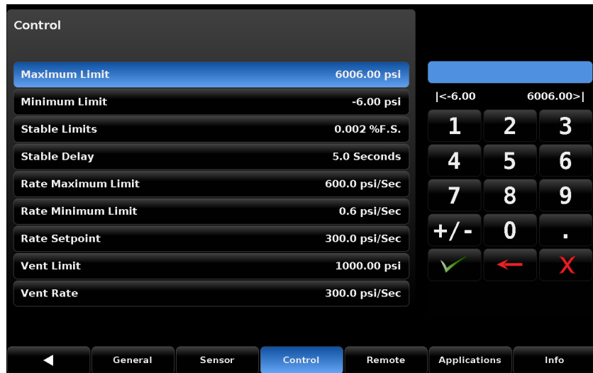
Figure 7.3.1 - Maximum Limit and Minimum Limit Buttons
