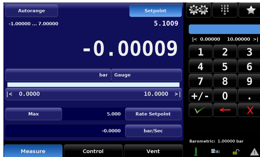
Figure 6.2.4 - Output Pressure Setpoint
