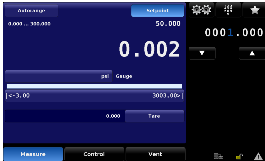
Figure 6.2.6.4 - Digital Step Screen
