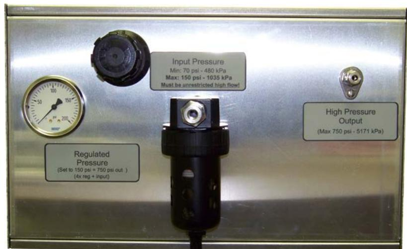
and the regulator knob is not fully counterclockwise. The input regulator filter provides basic filtering of large particles and liquids. It should periodically be checked for excessive contamination and emptied of liquids. **Note: The input pressure supply should have**
