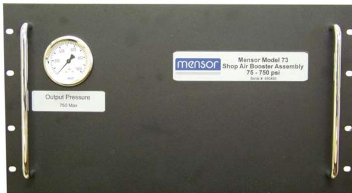
speed while still maintaining the output pressure, but at a slower recharge rate. The drive speed is adjusted by removing the top cover and adjusting the yellow ball valve lever. The unit is shipped with this lever in the wide open position. Experience has shown, that under all but the most extreme conditions, temperature problems should be of no concern.
