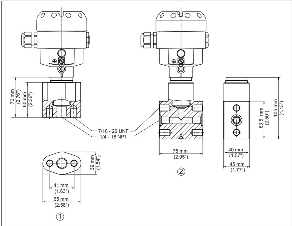
Fig. 54: CPT-2x, raccordement selon CEI 61518
