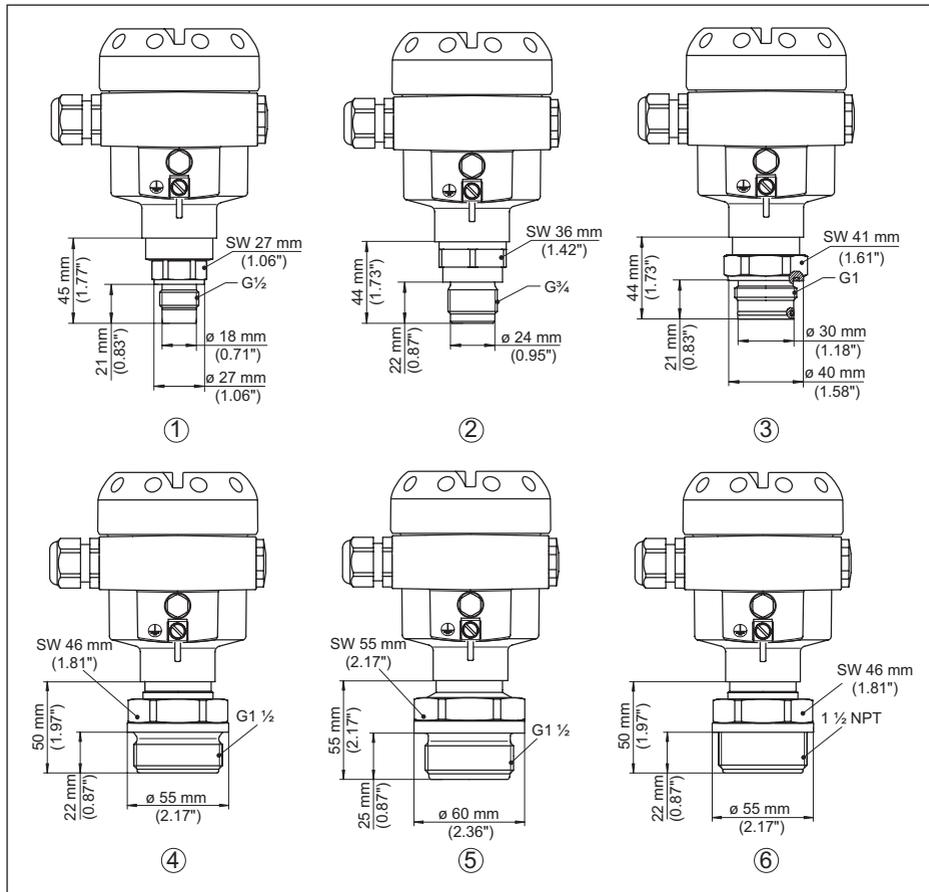
Fig. 50: CPT-2x, raccord fileté arasant
