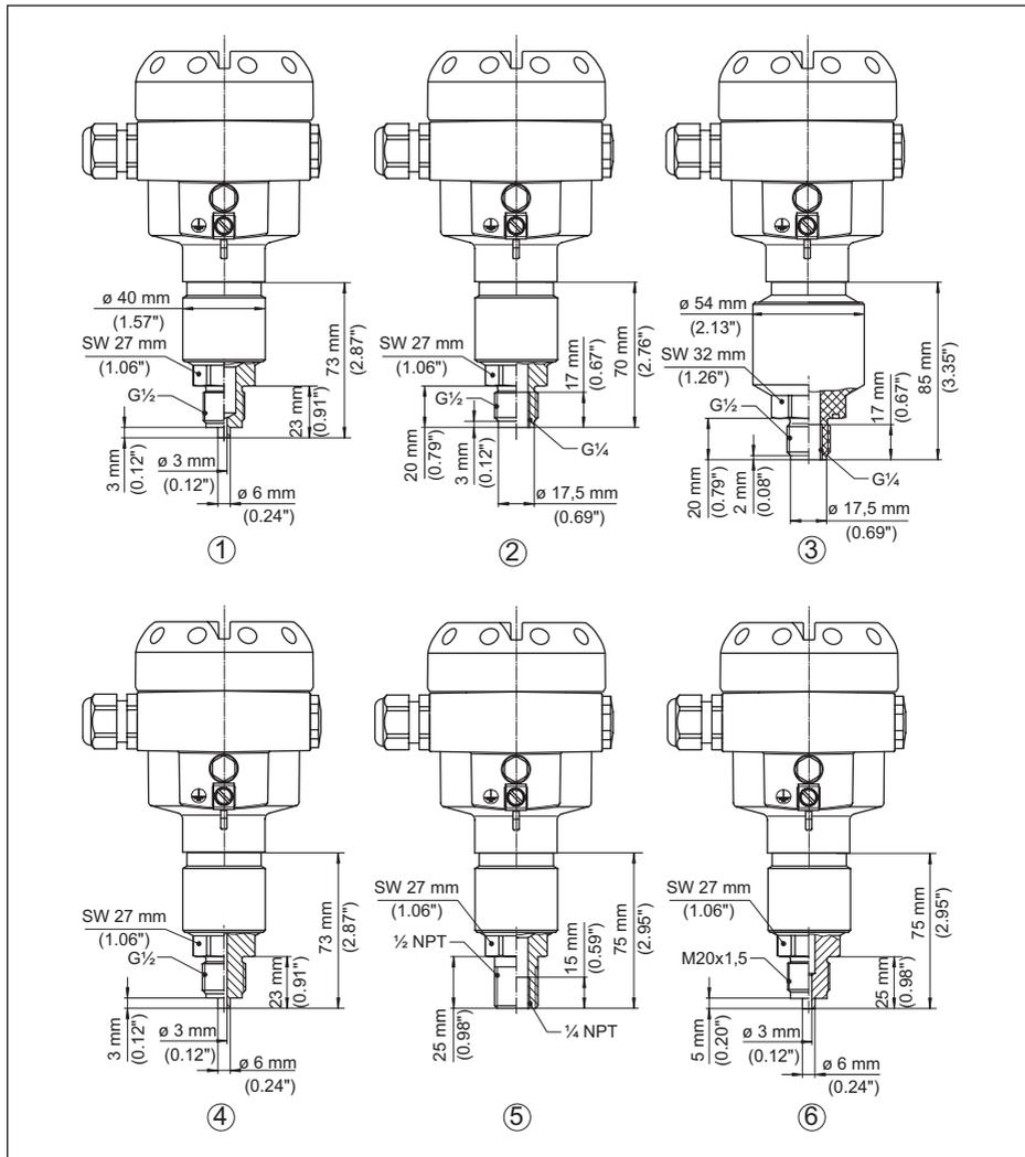
Fig. 49: CPT-2x, raccord fileté non arasant
