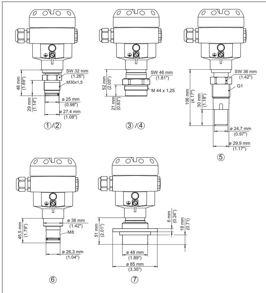
Fig. 53: CPT-2x, raccord à tube
