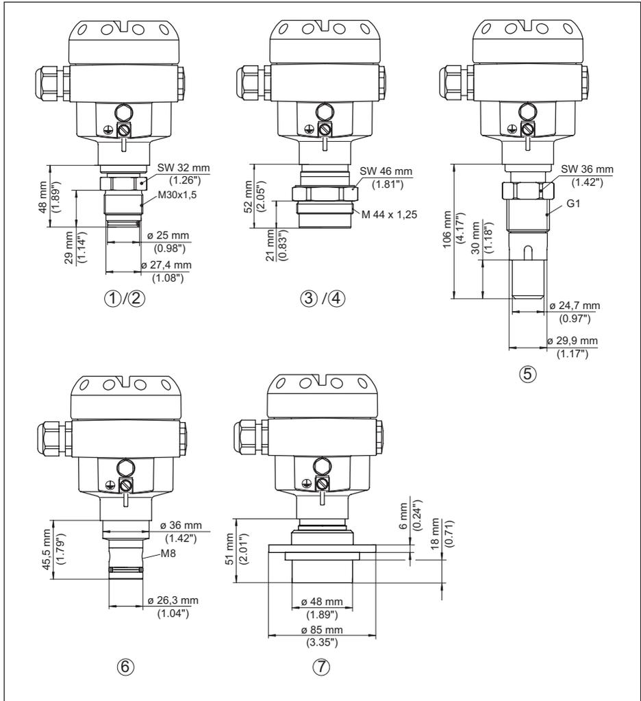
Fig. 54: CPT-2x, racor tubular
