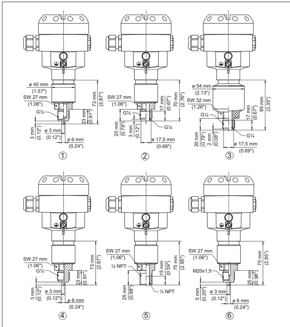
Fig. 50: CPT-2x, racor roscado no frontal rasante
