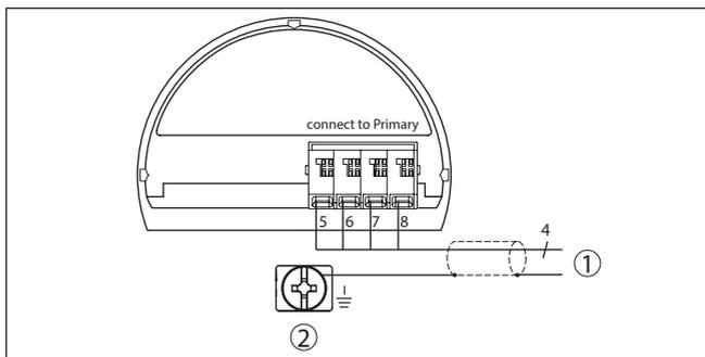
Fig. 25: Plan de raccordement CPT-2x appareil secondaire
