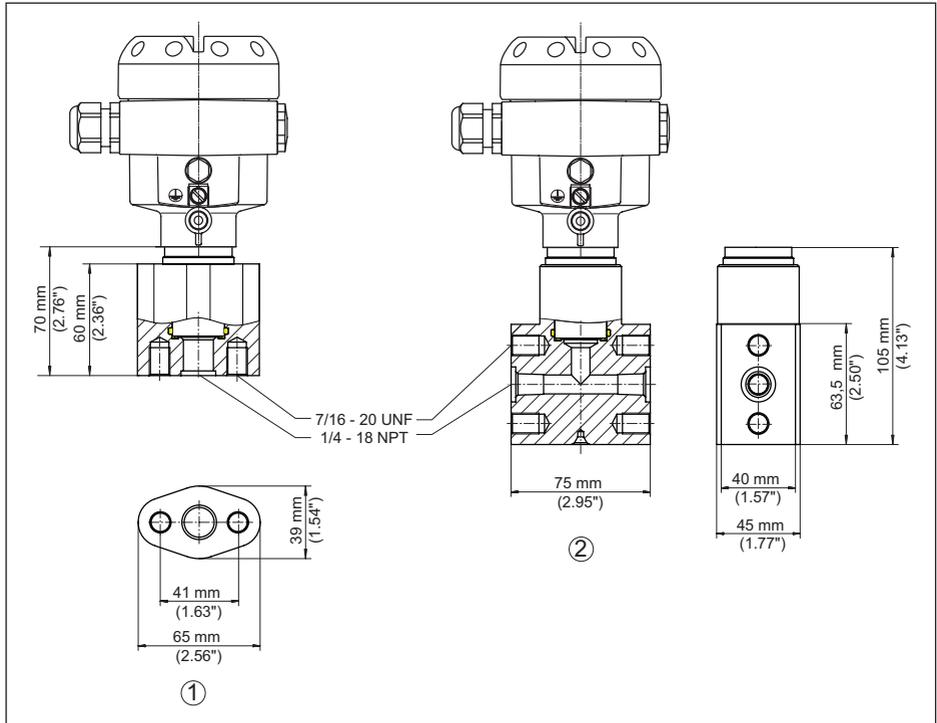
Fig. 43: CPT-2x, raccordement selon CEI 61518
