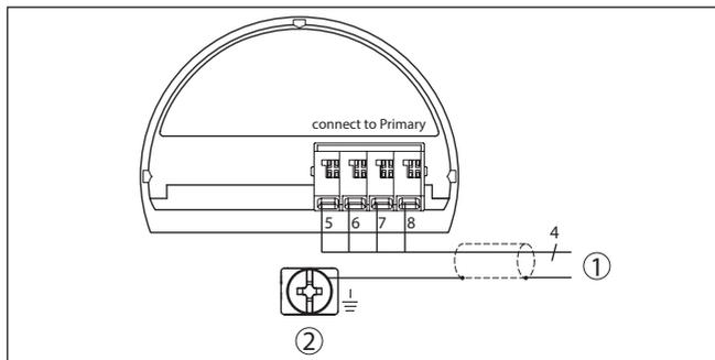
Fig. 21: Plan de raccordement CPT-2x appareil secondaire
