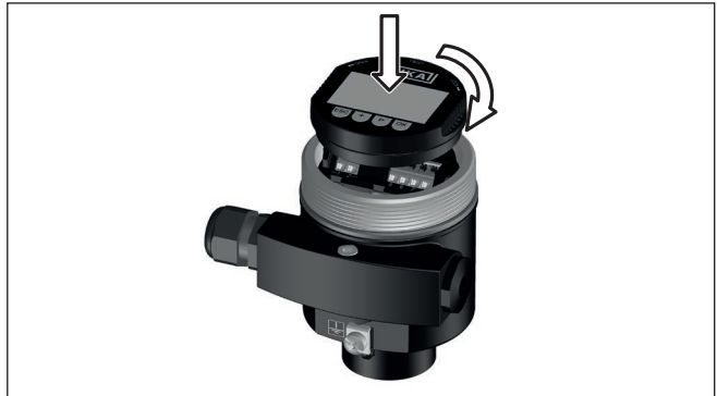
Fig. 24: Installing the display and adjustment module in the electronics compartment of the single chamber housing
