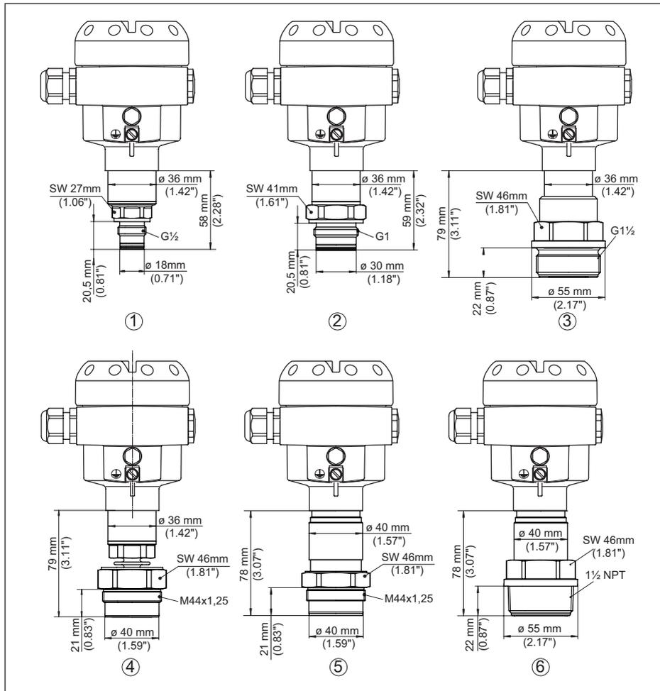
Fig. 49: IPT-2x, raccord fileté arasant
