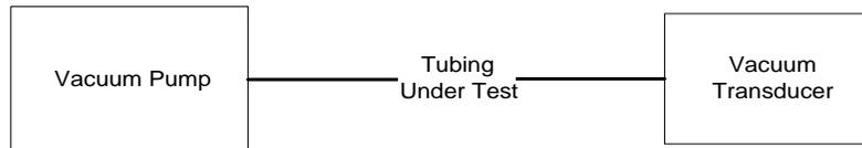
Figure 3. – Test Setup for Tubing Test
