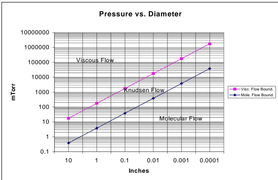
Figure 5. - Transitional Boundaries for Viscous and Molecular Flow
