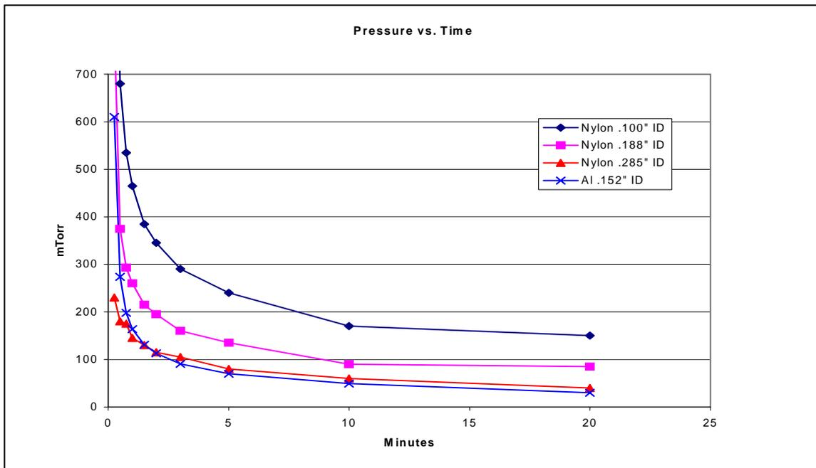
Figure 4. – Transducer Measurements on 48" Tubing Samples vs. Time
